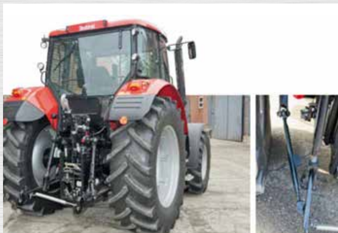
UK/Irish spec tractors come with a Dromone push-back hitch, while the ineffective stabilisers (right) can be replaced by Walterscheid options. Mudguards are scheduled for strengthening.
