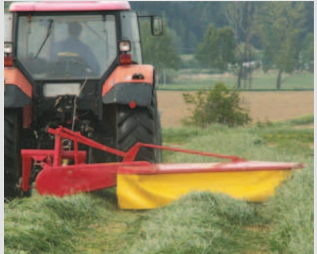
The location of heavy blades on large diameter drums creates very high blade speed, efficiently cutting just about any type of grass or forage. The drums are precisely balanced for a smooth, vibration-free run.
