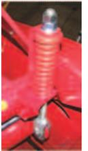
The breakaway safety system protects the mower when a drum hits an obstacle.
