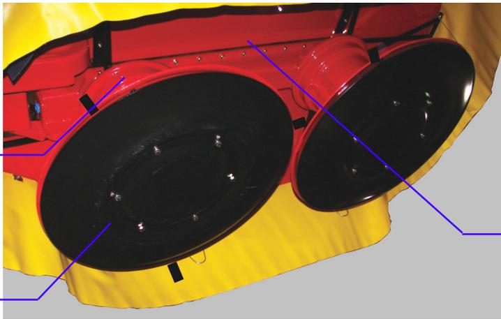
Drums are driven by a heavy duty gearbox equipped with quiet bevel gears. Simple gearbox design with a minimum number of moving parts is one of the features that make this mower virtually maintenance-free. The gearbox is filled with grease, rather than oil, eliminating any chances of leaks and allowing the mower to work on slopes. The high location of the gearbox also protects it from mechanical damage.
