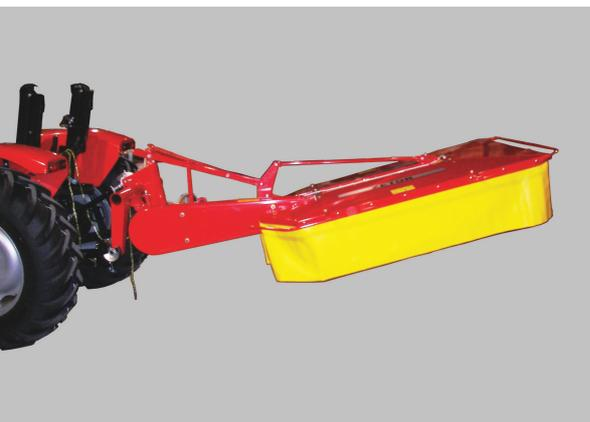
The metal hood resists abuse as well as heavy snow during winter storage. Metal rails around the safety curtain protect the most exposed areas of the curtain, extending its life considerably. Switching from working to transport position is effortless and does not use any hydraulic cylinder (tractor does not need hydraulic outlets).
